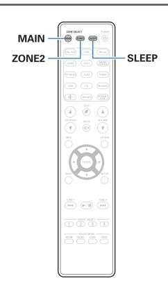
You can have the power automatically switched to standby once a set time has elapsed. This is convenient for viewing and listening while going to sleep. The sleep timer function can be set for each zone.
