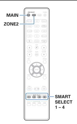
Settings such as the input source, volume level and sound mode can be registered to the SMART SELECT 1 - 4 buttons.
